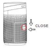
4. Put the filter into the machine.
